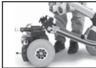
Figure 22. Separating The Frame Sections
